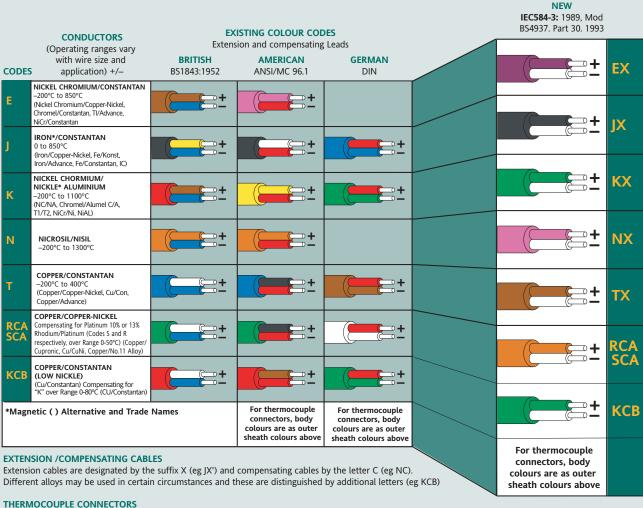
New colour coded connectors are marked IEC and have a grey body with a clearly visible colour coded area (with exceptions of the fascia/panels sockets). This is to prevent any confusion regarding the use of the new and old colour coded connectors
